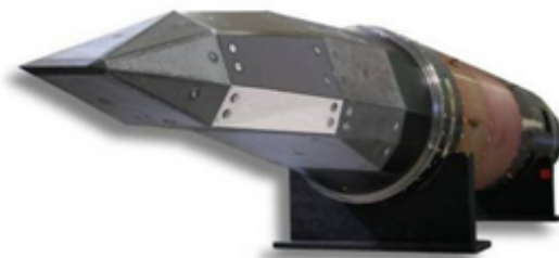
Figure 4.9: SHEFEX I re-entry body with faceted TPS.
